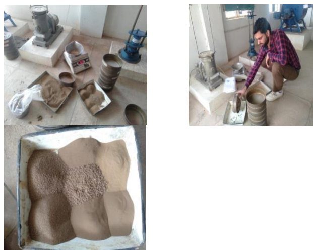
Fig. 3: Sieve analysis at civil engineering lab Dr. C V Raman University
